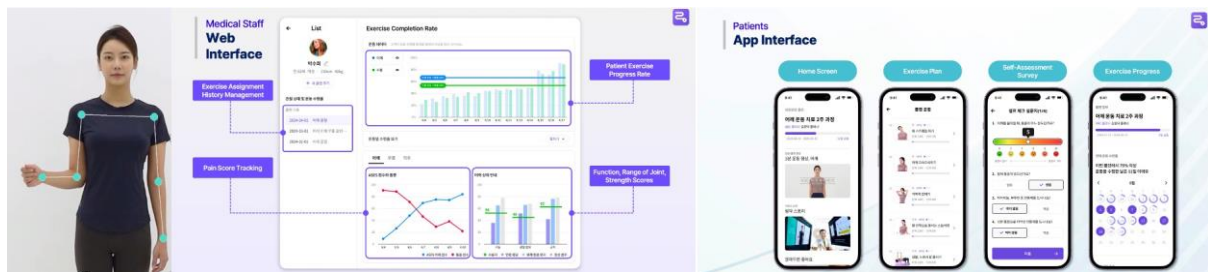
Fig. 3. A company utilizes machine learning-based pose estimation technology to measure a patient's range of motion, analyze the patient's current condition based on the results, and assign the most suitable rehabilitation exercises. This figure is used with permission from Itphy, Inc.
