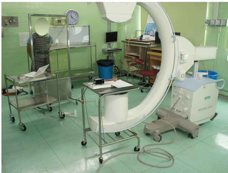
Fig. 1. Experimental setting. The motor–humerus complex was positioned on a radiolucent table under a C-arm. Using the rotation device, the proximal part was rotated, while the cut distal part was fixed. A fluoroscopic image was taken at each consecutive rotational position.
